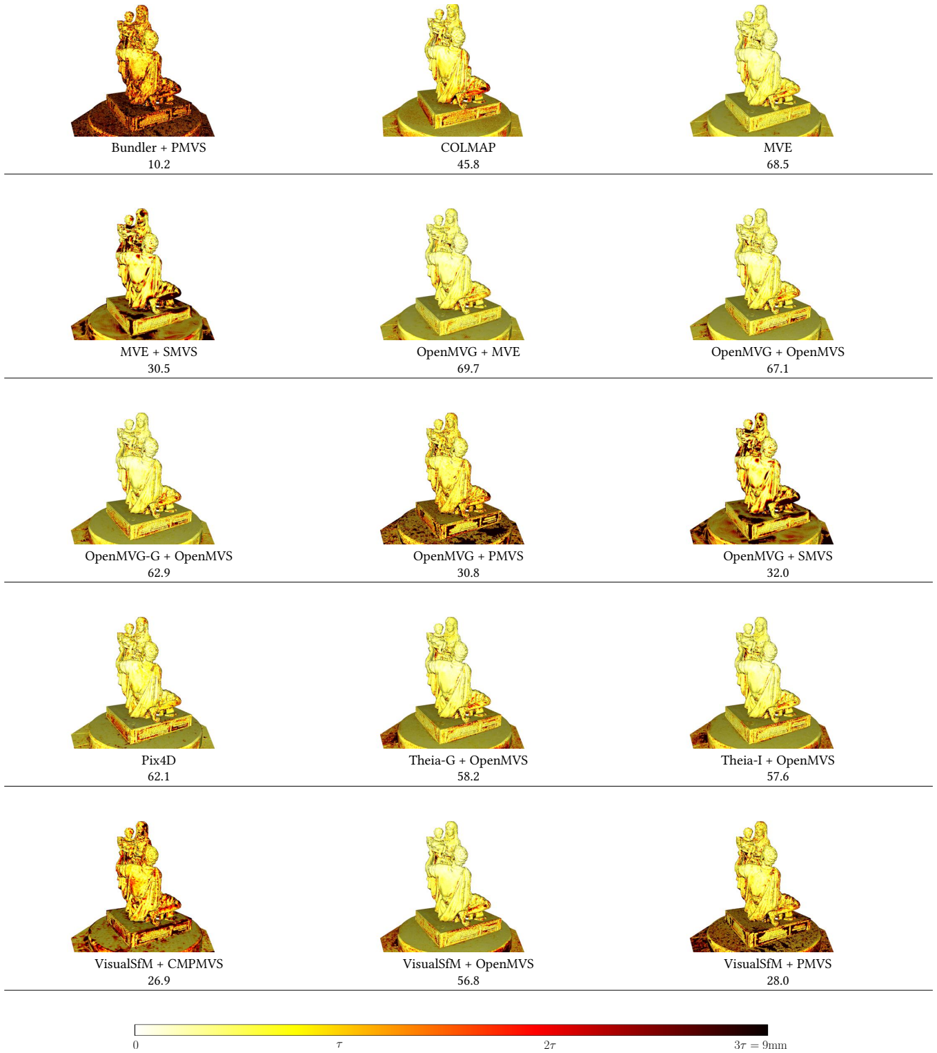
Figure 2. Family dataset. For each technique, we show the ground-truth point set, with distance to the reconstructed model coded by color. The number listed for each technique is R(\tau) .
