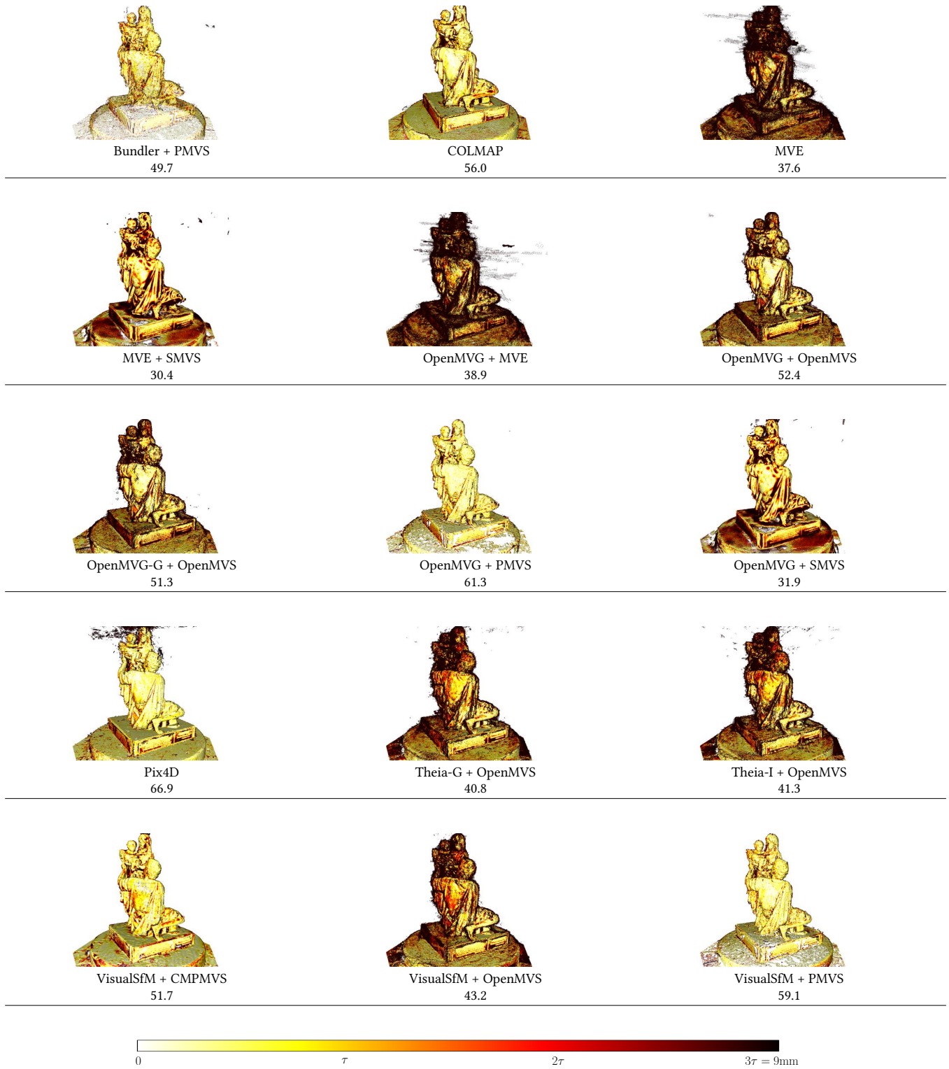
Figure 1. Family dataset. For each technique, we show the reconstructed point set, with distance to the ground-truth model coded by color. The number listed for each technique is P(\tau) .
