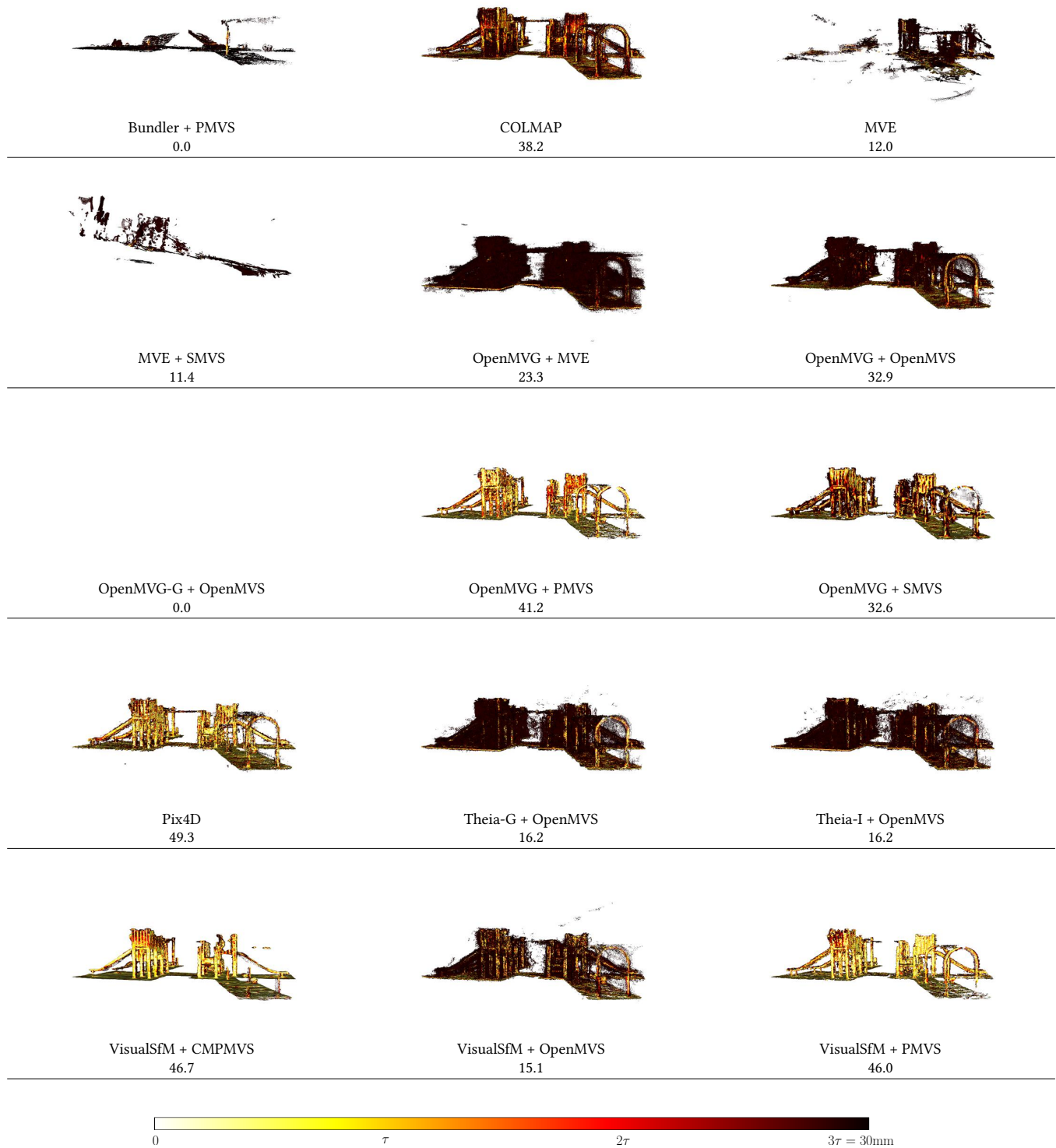
Figure 13. Playground dataset. For each technique, we show the reconstructed point set, with distance to the ground-truth model coded by color. The number listed for each technique is P(\tau) .
