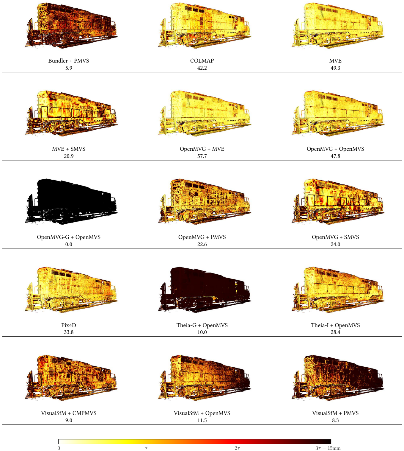
Figure 16. Train dataset. For each technique, we show the ground-truth point set, with distance to the reconstructed model coded by color. The number listed for each technique is R(\tau) .
