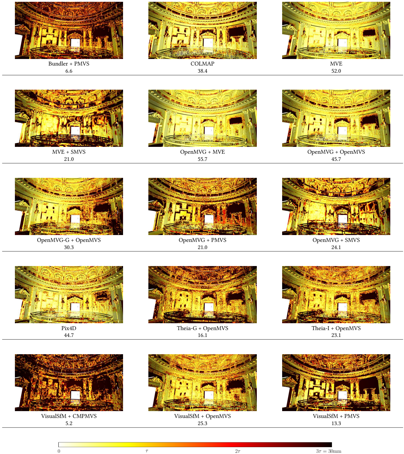
Figure 24. Museum dataset. For each technique, we show the ground-truth point set, with distance to the reconstructed model coded by color. The number listed for each technique is R(\tau) .
