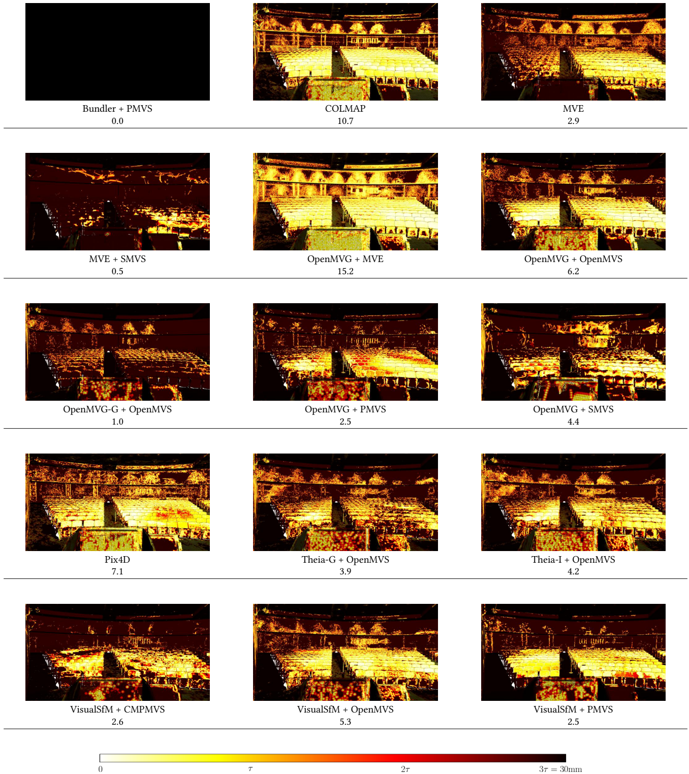
Figure 18. Auditorium dataset. For each technique, we show the ground-truth point set, with distance to the reconstructed model coded by color. The number listed for each technique is R(\tau) .
