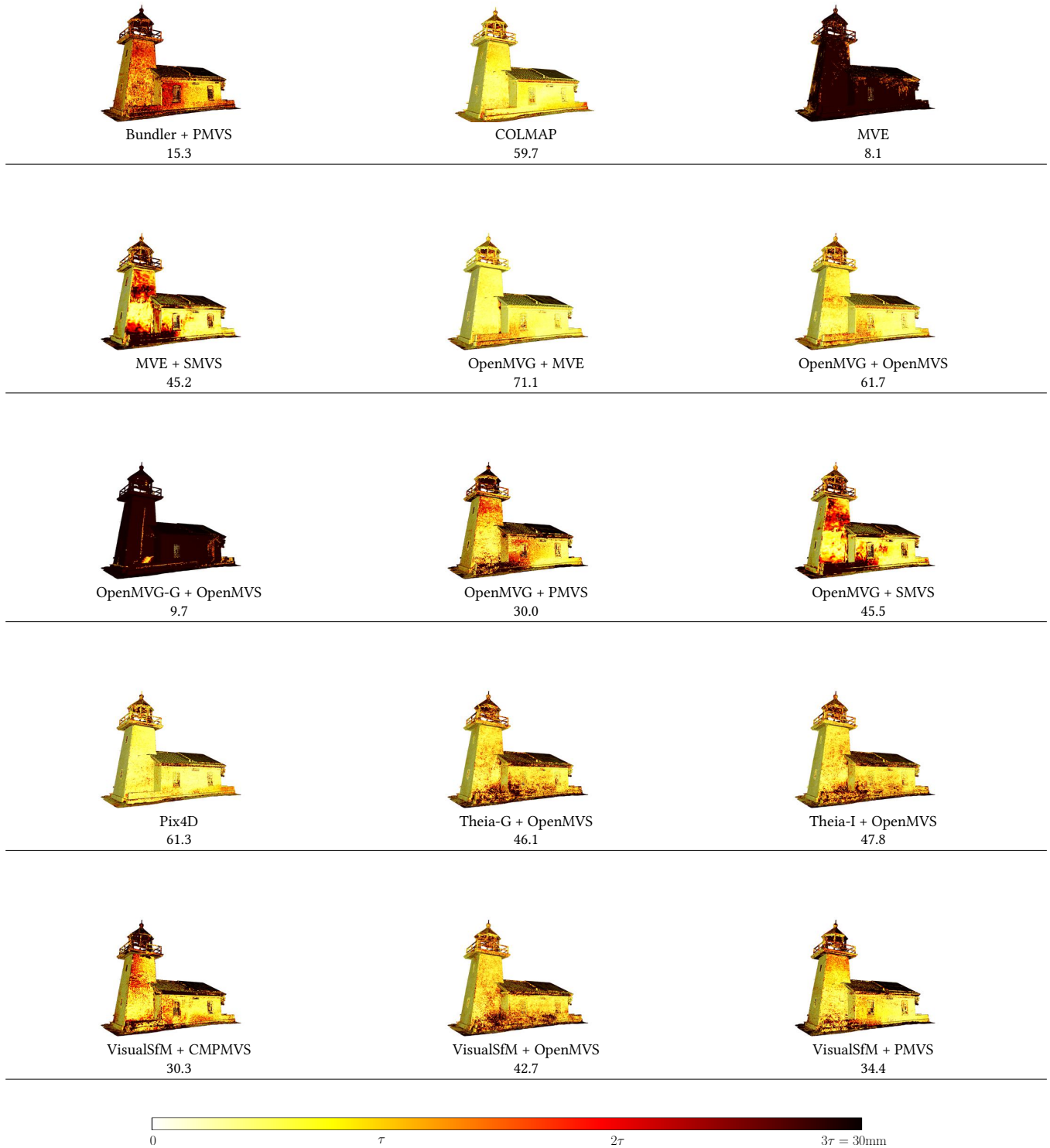
Figure 8. Lighthouse dataset. For each technique, we show the ground-truth point set, with distance to the reconstructed model coded by color. The number listed for each technique is R(\tau) .
