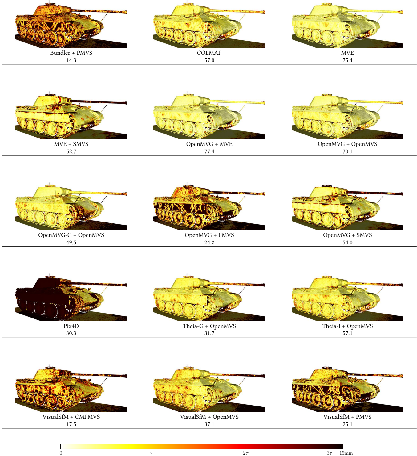
Figure 12. Panther dataset. For each technique, we show the ground-truth point set, with distance to the reconstructed model coded by color. The number listed for each technique is R(\tau) .
