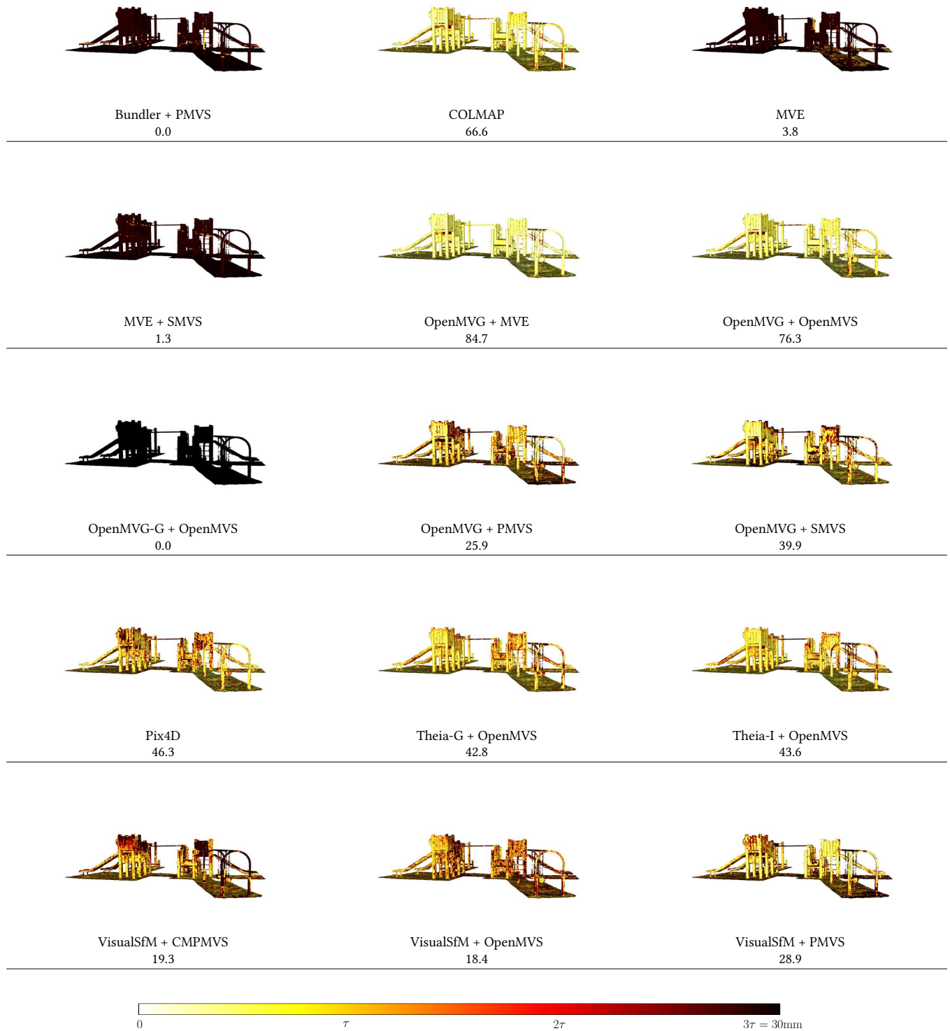
Figure 14. Playground dataset. For each technique, we show the ground-truth point set, with distance to the reconstructed model coded by color. The number listed for each technique is R(\tau) .
